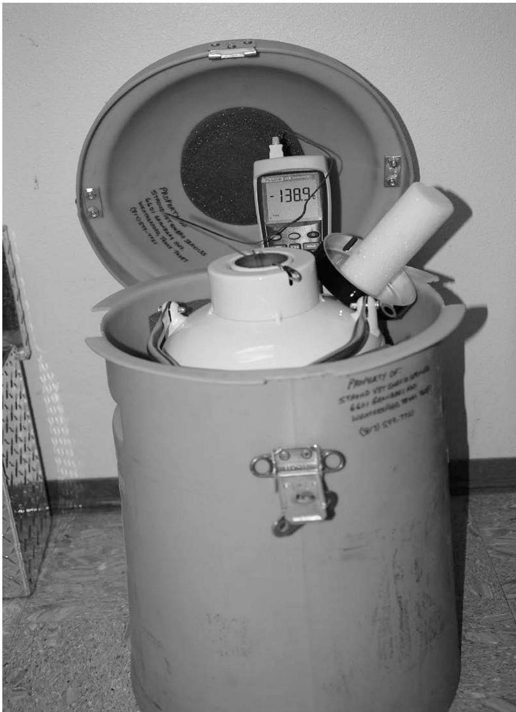
**Figure 2.** Dry shipper 10 days post charging with liquid nitrogen. Temp  $-138.9^{\circ}\text{C}$
